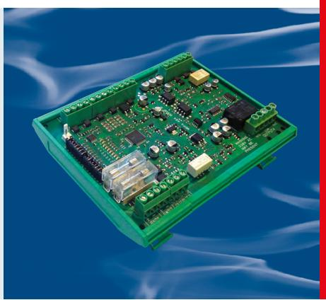
The Protec 4 way input/output interface is a auxiliary powered input / output device providing 2 local zones of conventional detectors, 2 monitored inputs, 2 local monitored alarm outputs and two volt free changeover contacts. The contacts may be used to connect to ancillary equipment.
